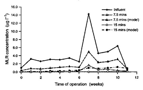
Pilot plant trials investigating anatoxin-a removal by GAC showed no breakthrough, whereas modelled results for the same operating conditions predicted breakthrough (UK WIR, 1995). This suggested that biological activity was also important for anatoxin-a removal by GAC.
