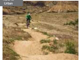
PBR Trail: Small/gentle rollers and berms, shape supported with rock materials, lots of undulations and meanders, flow adjusted to reduce speeds (to reduce breaking, sliding), soil amendments for tread shaping
