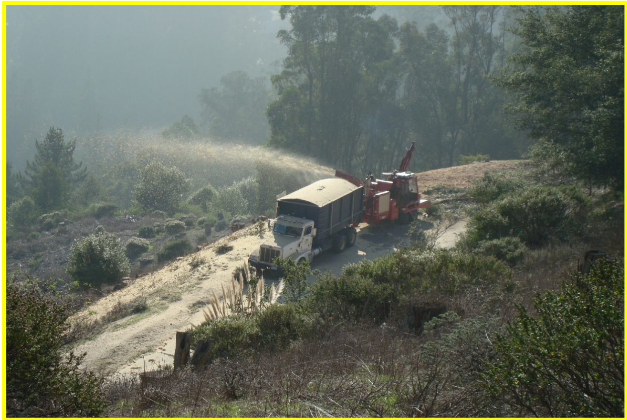
Creating fuel break using wood chipper
